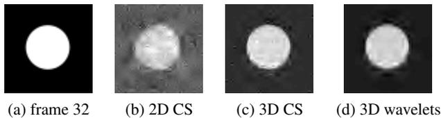
**Fig. 3.** (a) Frame 32 of a 64-frame video sequence ( $64 \times 64$  images of a disk moving from top to bottom, corresponding to 262,144 3-D voxels). (b) CS frame-by-frame reconstruction using 20,000 total 2-D random projections (313 independent 2-D projections for each image in the sequence). (c) Full 3-D video reconstruction from 20,000 3-D random projections (using 3-D wavelets as the sparsity-inducing basis). (d) Result of 3-D wavelet thresholding to 2000 total coefficients.
