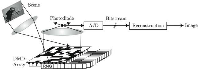
**Fig. 1.** Compressive Imaging (CI) camera block diagram. Incident light field (corresponding to the desired image  $x$ ) is reflected off a digital micromirror device (DMD) array whose mirror orientations are modulated in the pseudorandom pattern  $\phi_m$  supplied by the random number generators (RNG). Each different mirror pattern produces a voltage at the single photodiode that corresponds to one measurement  $y(m)$ .
