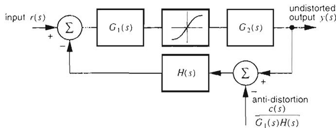
Fig. 8. Feedback amplifier with antidistortion moved to output side of feedback factor.
