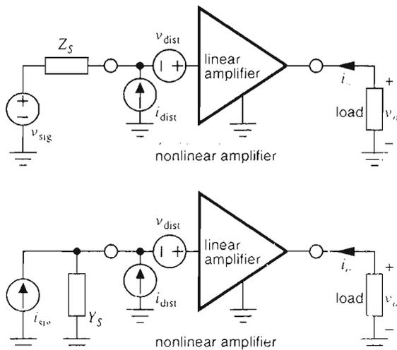
Fig. 10. Distortion generators at input of amplifier with Thévenin and Norton representations of signal source.
