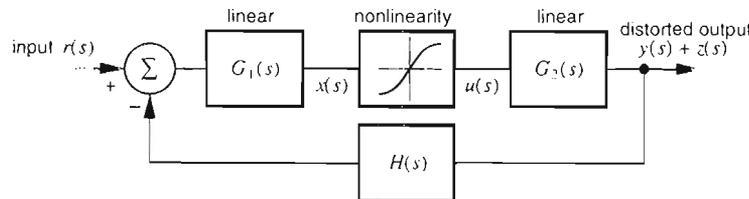
Fig. 3. Feedback amplifier with static nonlinearity in its forward path.
