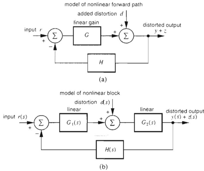
Fig. 1. Simplistic representations of nonlinear distortion in feedback amplifier. It is assumed that the input signal is adjusted so that the output amplitude remains constant when any change to the circuit is contemplated. (a) Basic. (b) Somewhat more realistic.
