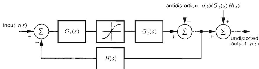
Fig. 9. Feedback amplifier with antidistortion inserted at two points.
