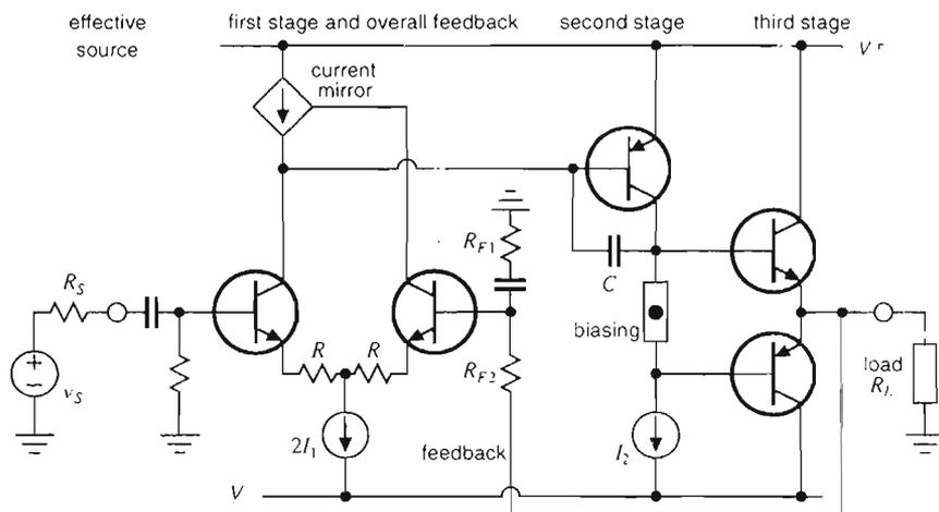
Fig. 11. Typical circuit topology for audio power amplifier.
