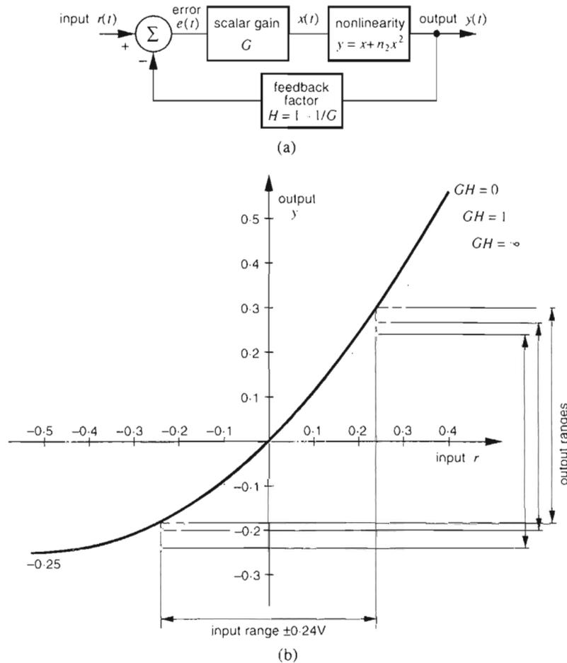
Fig. 2. Nonlinear feedback system and its transfer characteristic for various values of loop gain.
