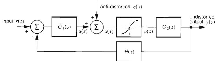
Fig. 4. Amplifier with antidistortion injected at the input of a static nonlinearity to give undistorted output.
