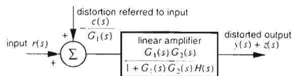
Fig. 7. Amplifier with distortion referred to its input.
