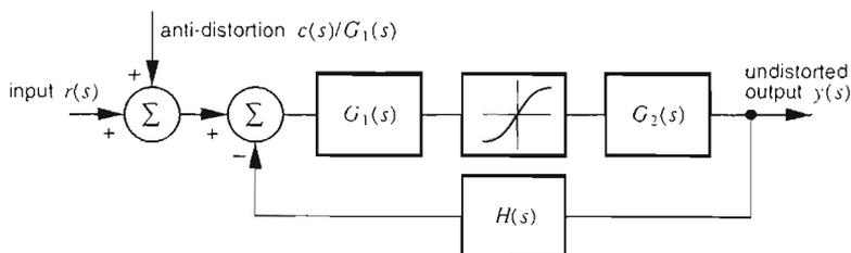
Fig. 5. Amplifier with antidistortion moved to its input.
