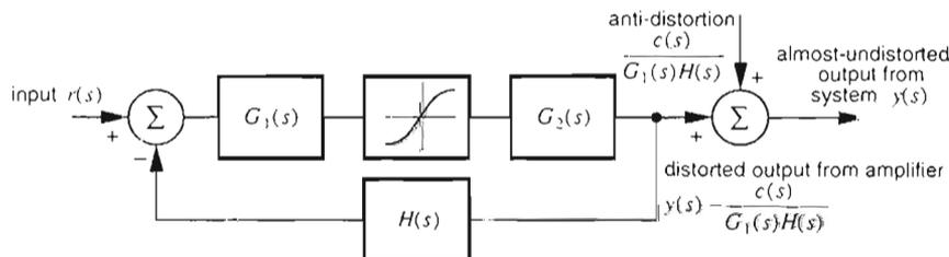
Fig. 6. Approximate equivalent of Fig. 4, based on the fact that amplifier with feedback is almost linear. Distortion values shown are based on large loop-gain approximation  $A(s) \approx 1/H(s)$ .
