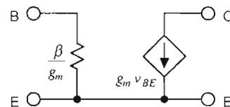
Fig. 12. Assumed small-signal equivalent circuit of BJT.
