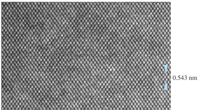
Figure 1.1 Image of silicon crystal obtained by transmission-electron microscopy.
