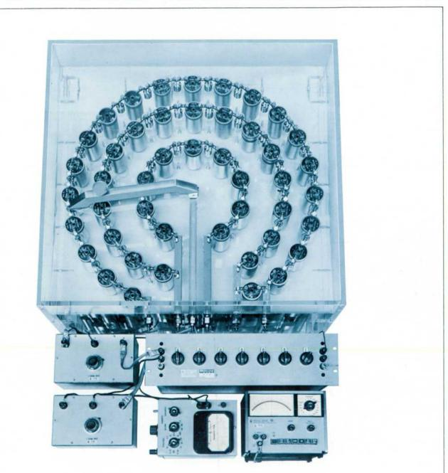
1.5 X 10-8 ACCURACY DC VOLTAGE COVER: DIVIDER USING NEW -hp- STANDARD RESISTORS, p. 8
