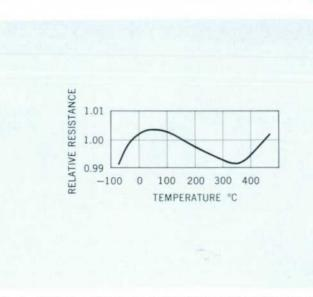
Fig. 4. Variation of resistance of resistance wire with temperature.
