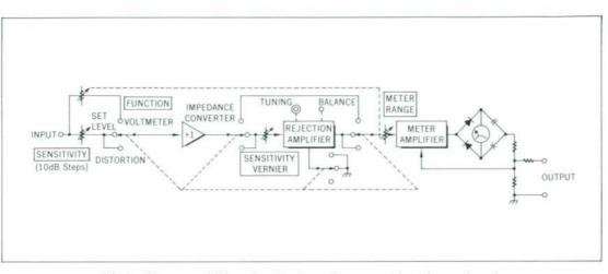
Fig. 3. Elements of Distortion Analyzer. Instrument functions as broadband calibrated ac voltmeter in 'Voltmeter' mode and as signal level indicator in 'Set Level' mode. In 'Distortion' mode, Rejection Amplifier can be tuned to suppress fundamental frequency of input signal, permitting comparison of distortion components level to total signal level.
