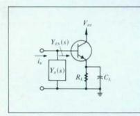
Fig. 1. Emitter follower with a capacitive load.
