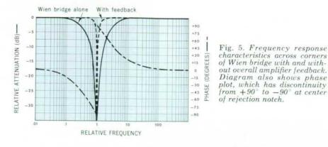
line in Fig. 5. As shown, the phase of the residual signal across the corners of the bridge lags the driving signal by 90°, if the bridge is tuned slightly below the signal frequency, and leads by 90° if the bridge is tuned above. A phase-sensitive detector therefore is able to sense any mistuning and indicate the direction that a correction should take.
