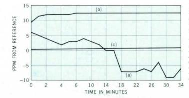
Fig. 6. Changes in resistance values of standard resistors at power level of 0.1 W. (a) Rosa-type resistor before cleaning of header. (b) Same resistor after header was cleaned, showing that many transient effects are caused by electrochemical cell formed on header by impurities. (c) -hp- type (Serial No. 0018) after two years service, showing that contamination has been eliminated by use of inert materials. (Note expanded time scale for first 6 minutes.)
