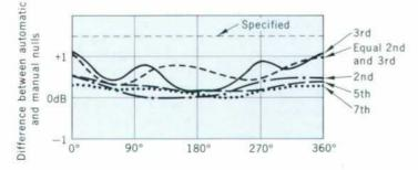
Fig. 7. Possible differences between manual and automatic nulling depth resulting from phase displacement of odd harmonics. Majority of differences are less than 1 dB and in practice, seldom exceed 1/2 dB.
