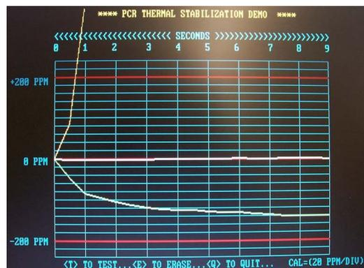
Figure 4. 9 seconds recording of 3 thermal transients - comparison of 3 technologies: Thick film (top). Thin film (bottom) and Double Sided Z foil (center)
