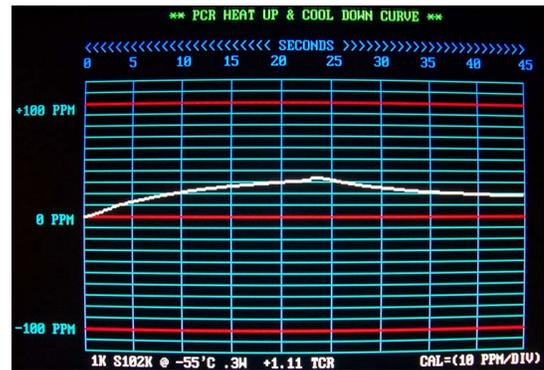
Figure 1. Continuous recording of  $\Delta R/R_{REF}$  during 45 seconds with power applied during the first 22 seconds.
