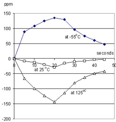
Figure 2. Recording of  $\Delta R/R_{REF}$ , S102C resistor, pulse 22/45sec, at 3 ambient temperatures:  $-55^{\circ}\text{C}$ ,  $25^{\circ}\text{C}$  and  $125^{\circ}\text{C}$ .
