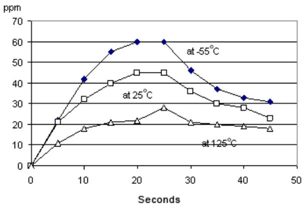
Figure 3. Recording for 45 seconds of  $\Delta R/R_{REF}$ , S102K style resistor, 0.6W pulse applied for 22 sec, at three ambient temperatures:  $-55^{\circ}\text{C}$ ,  $25^{\circ}\text{C}$  and  $125^{\circ}\text{C}$ .
