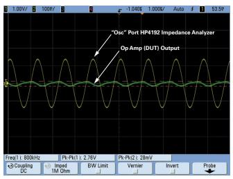
Figure 5. Probed outputs of HP4192A "Osc" output port and op amp output pin.
