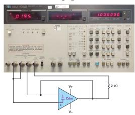
Figure 3. Direct C<sub>DM</sub> measurement method test setup.
