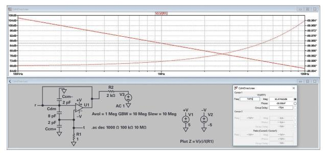
Figure 1. Direct measurement of  $C_{DM}$  impedance in LTspice. Plot V(r)/I(R1) to get the impedance. In this case, at 1 MHz, Z is 19.89437 k $\Omega$  (10<sup>65.97/20)</sup> at -89.996°, which is exactly 8 pF using C = 1/( $2\pi \times Z \times Freq$ ).
