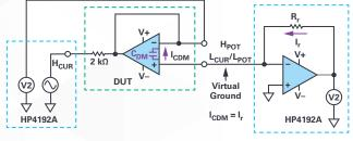
Figure 2. Test circuit for C<sub>DM</sub>.
