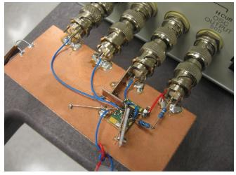
Figure 4. The HP4192A setup showing the board. Excitation through 2 k $\Omega$  and voltage readback are on the right. The DUT used is an LT1792 8-lead SO on a single postage stamp LB2223. TIA is on the left, internal to HP4192A.
